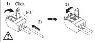
Ensure the wire is stripped to Max. 8mm and all wires are fully inserted into the terminal block end with no loose strands left outside.
