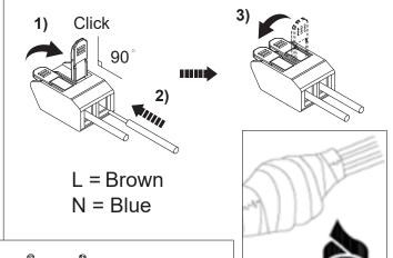
**IMPORTANT**: Cover the connections with two layers of good quality electrical insulation tape, extending at least 3cm beyond the cable entry side of the connector block. Wiring must be completed by qualified electrician. Good quality electrical insulation tape can be purchased from any DIY retailer.
