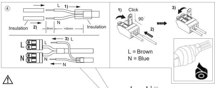
**IMPORTANT**: Cover the connections with two layers of good quality electrical insulation tape, extending at least 3cm beyond the cable entry side of the connector block. Wiring must be completed by qualified electrician. Good quality electrical insulation tape can be purchased from any DIY retailer.
